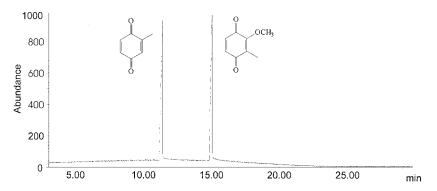
FIG. 3. Reconstructed gas chromatogram from GC-MS analysis of a dichloromethane extract of secretion from a male *Orthoporus dorsovittatus* (fused silica column, 30 m  $\times$  0.22 mm, coated with DB-5; oven temperature: 40°C for 4 min and raised 8°C/min to 270°C).
